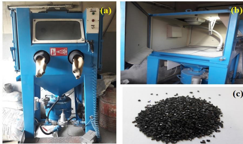
Fig.3.1. (a) Front and (b) side view of shot blasting machine and, (c) Blasting medium (Virgin alumina).
