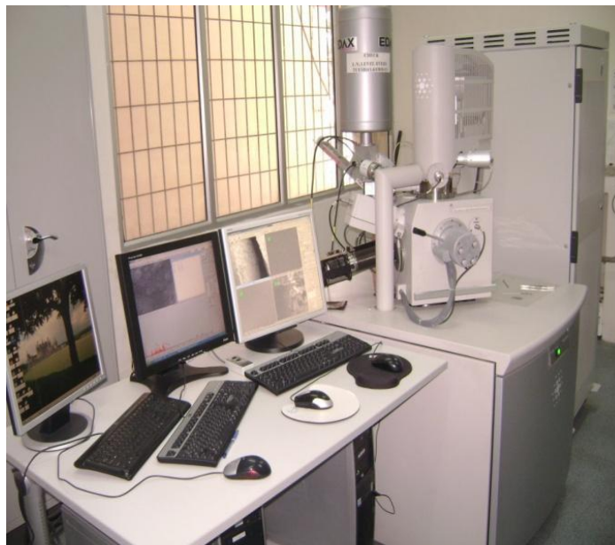
Figure A-3: Typical View of the Field Emission Scanning Electron Microscope (FE-SEM) Used for Microstructural Investigation
