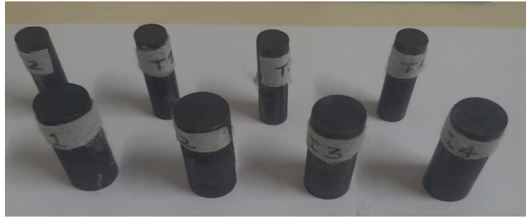
Fig. 3.3. The pin samples used for the pin-on-disc sliding wear test.
