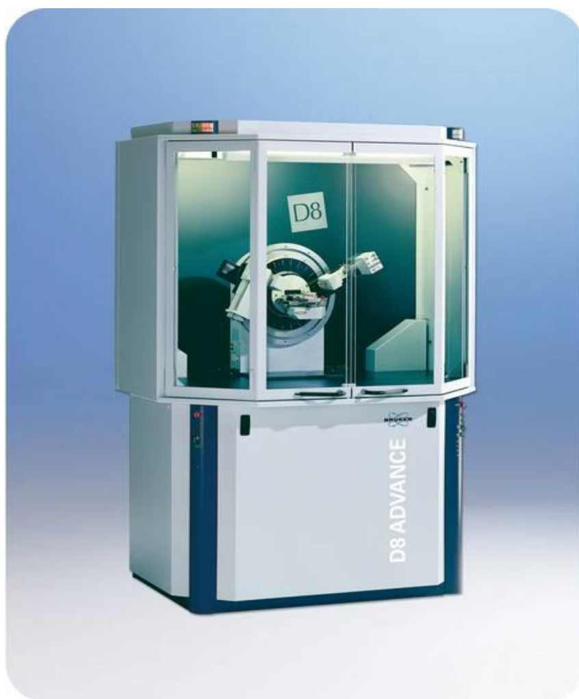
Figure A-1: View of the X-Ray Diffraction Equipment Used for Phase Analysis.
