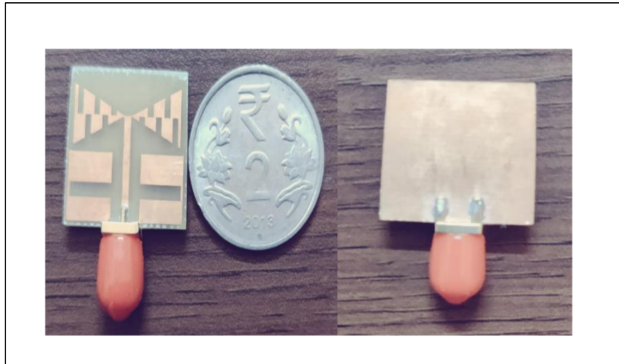
Figure 5.8: Fabricated prototype for the proposed antenna (Ant 2)
