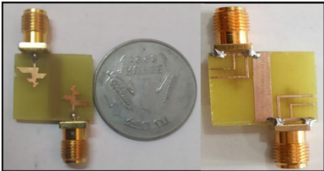
Figure 5.28: The image of the radiating patch and ground plane for the fabricated Ant IV (final proposed design) antenna compared with the size of a standard 1Re coin.
