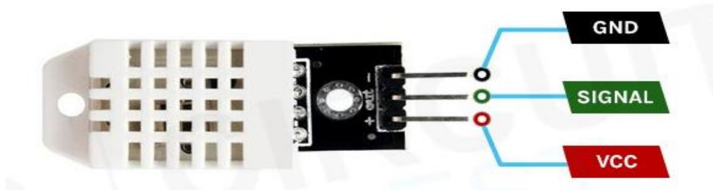
Figure 18: DHT22 Pin Layout
