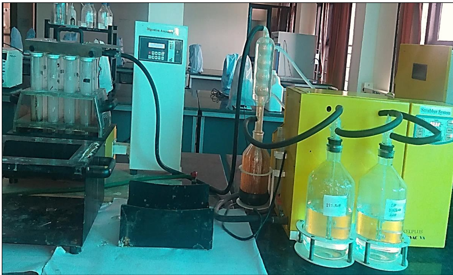
Figure 4.5 KEL PLUS assembly for digestion the sample
