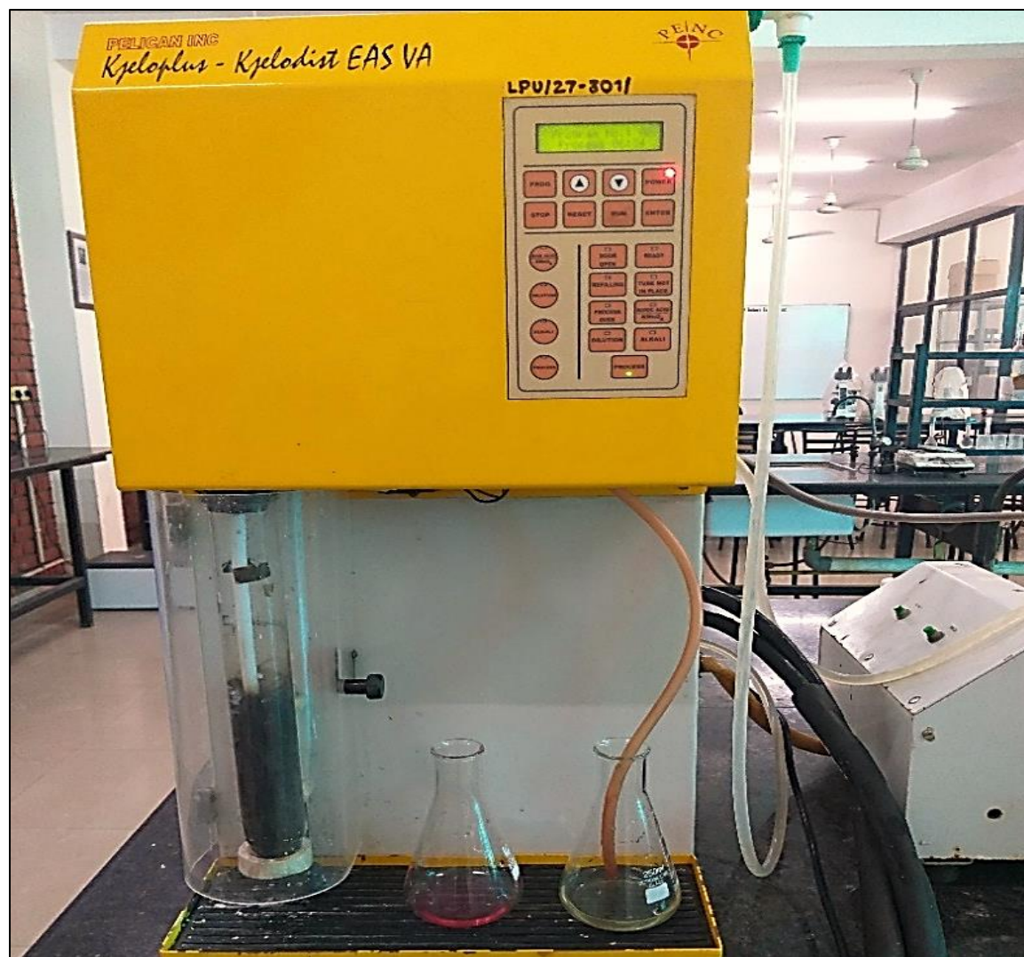
Figure 4.7 shows the KELPLUS distillation assembly
