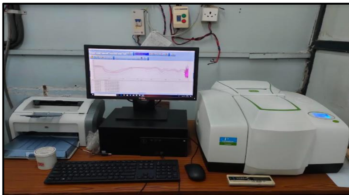
Figure 3. 16 Fourier Transform infrared spectrometer of UGC DAE CSR Center, Kolkata
