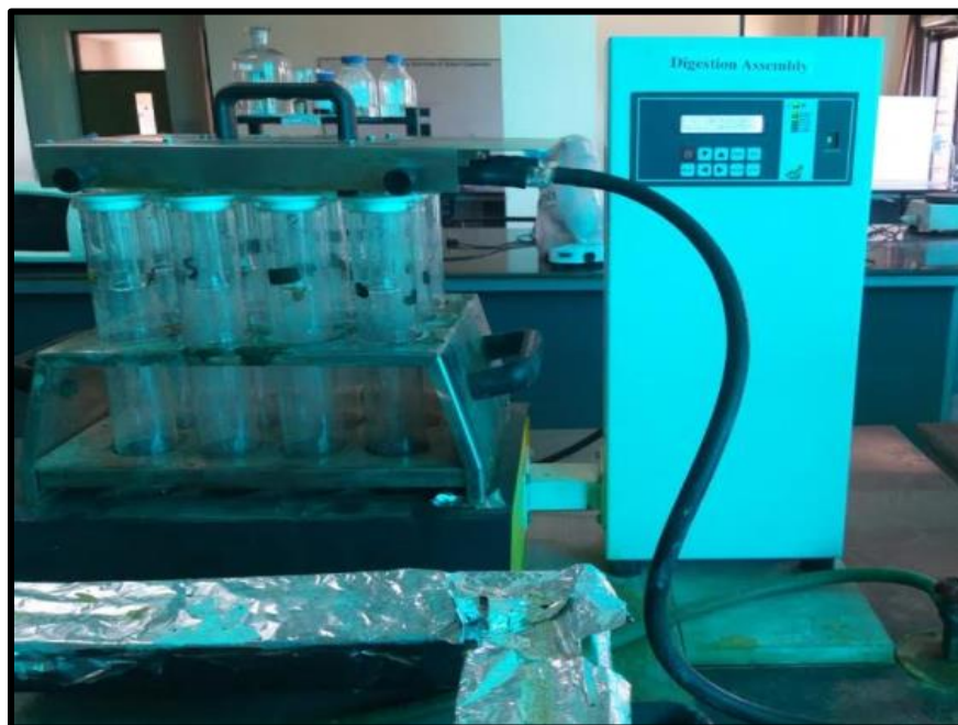
Figure 3. 8 Digestion unit for crude protein analysis
