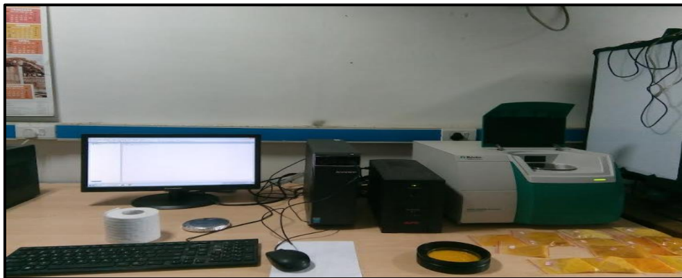
Figure 3. 14 Near infrared spectrometer of CSIR-CSIO Chandigarh laboratory
