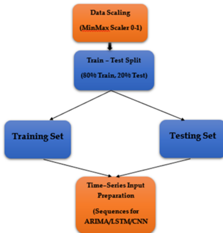
Figure 4.7 Data Scaling, Splitting, and Time-Series Input Preparation Pipeline
