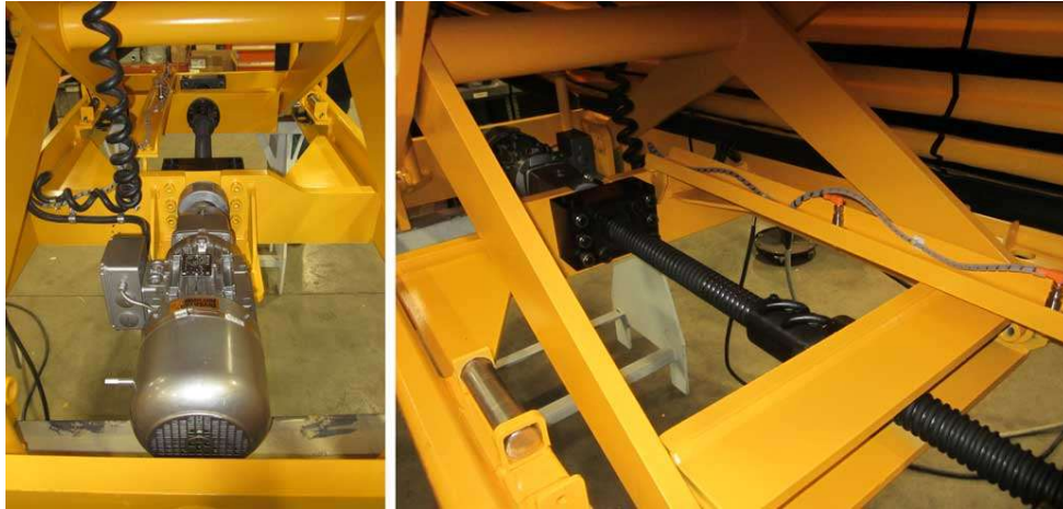
Figure 4.39. The Screw-jack scissor lift hybrid was used in the present experiment to lift the pool elevator.
