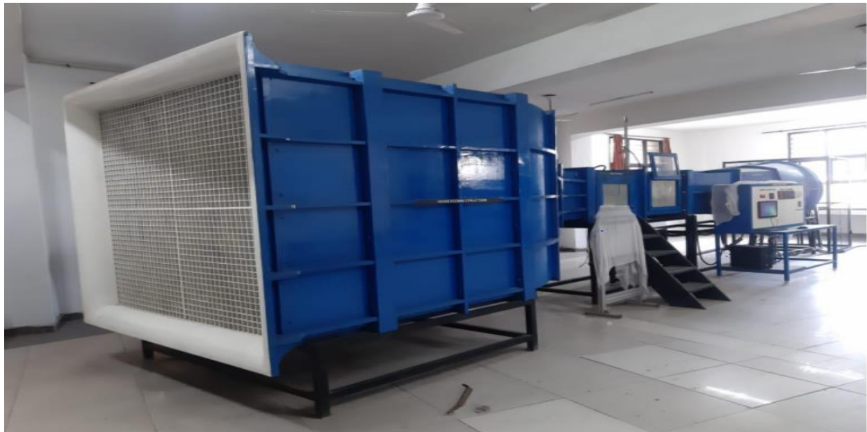
Fig 4-2 Subsonic wind tunnel with six-component force measurement set up and DAQ software for plotting the results
