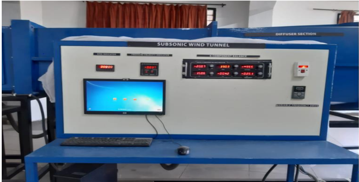
Fig 4-1 System with DAQ software for measuring six component forces
