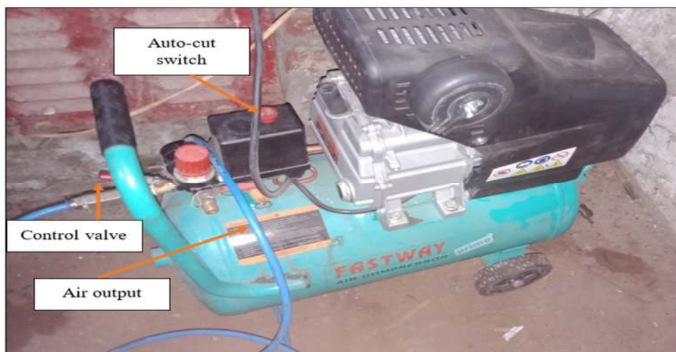
Fig 3.18 Air compressor used for compressed air supply
