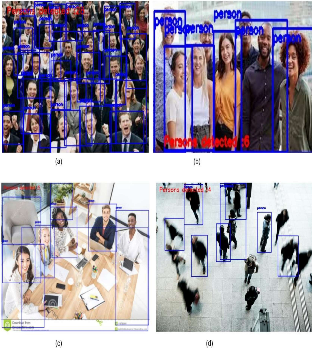
Figure 5.12 People detection and counting by vision node
