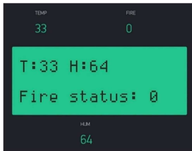
Figure 4.11 Blynk Dashboard Showing No Fire Detected
