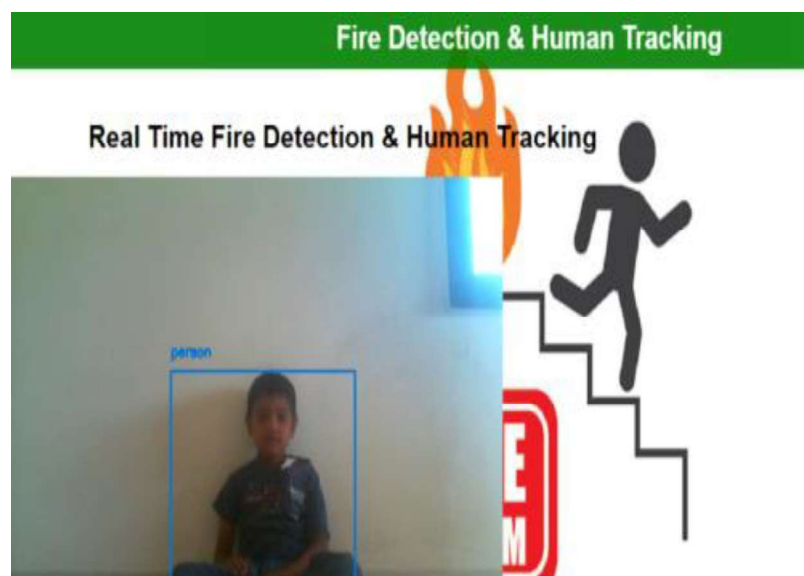
Figure 5.9 Real-time People Detection and Visualization On Web Application
