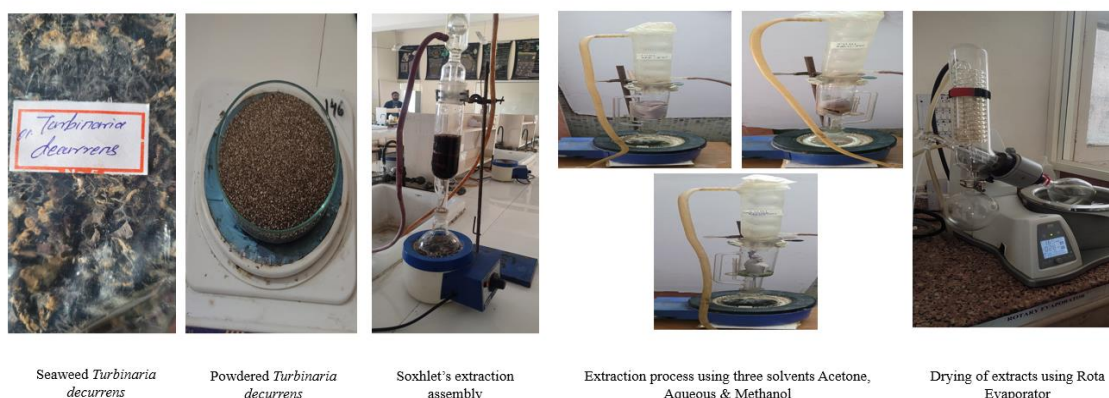
Figure 6: Extraction of phytochemical constituents by Hot percolation method using Soxhlet Extraction assembly and drying of solvent extracts using Rotary evaporator.
