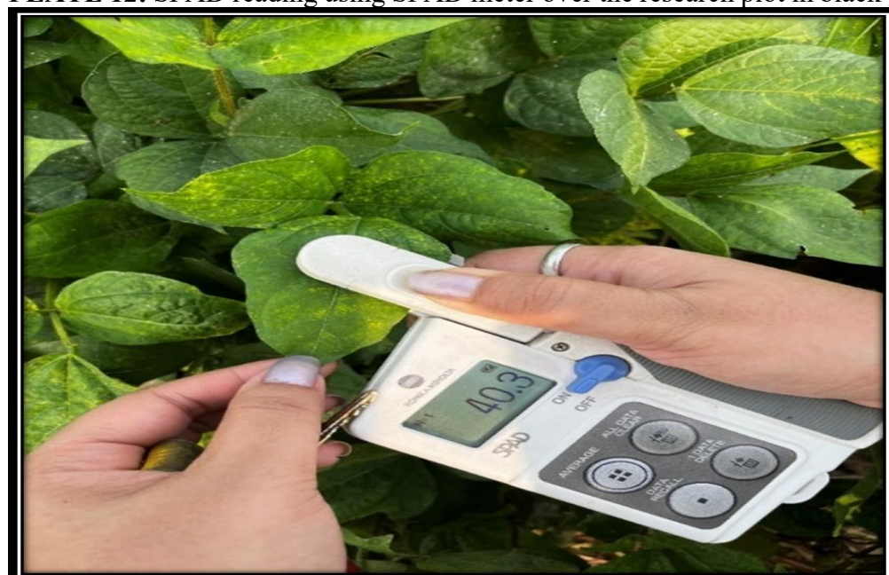
PLATE 12: SPAD reading using SPAD meter over the research plot in black gram
