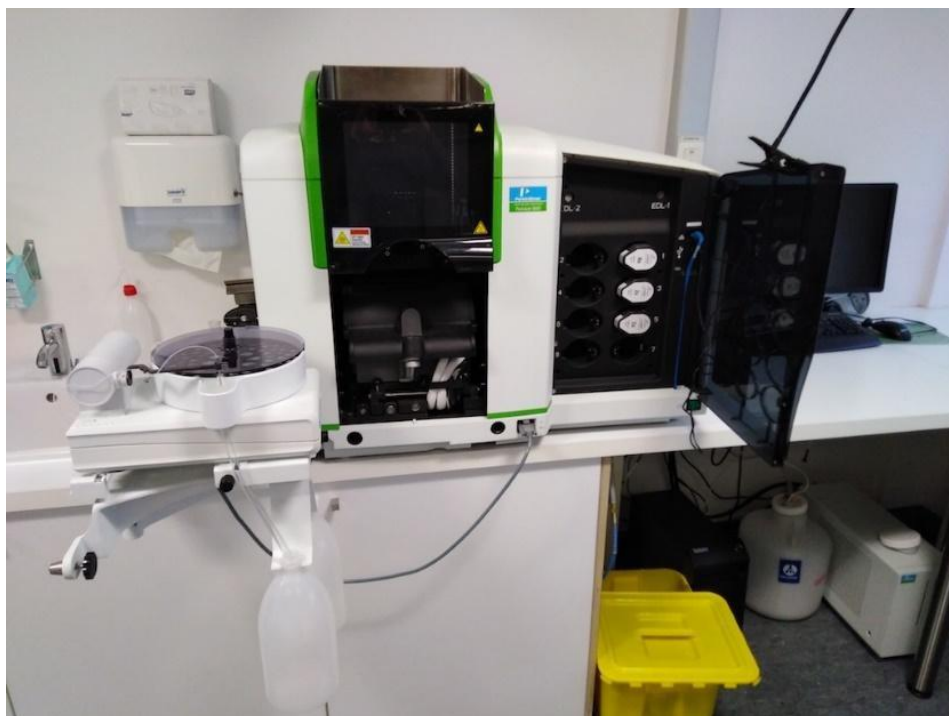
Figure 3.2: PerkinElmer PinAAcle 900T Atomic Absorption Spectrometer instrument for heavy metal analysis (Bionex Scientific)
