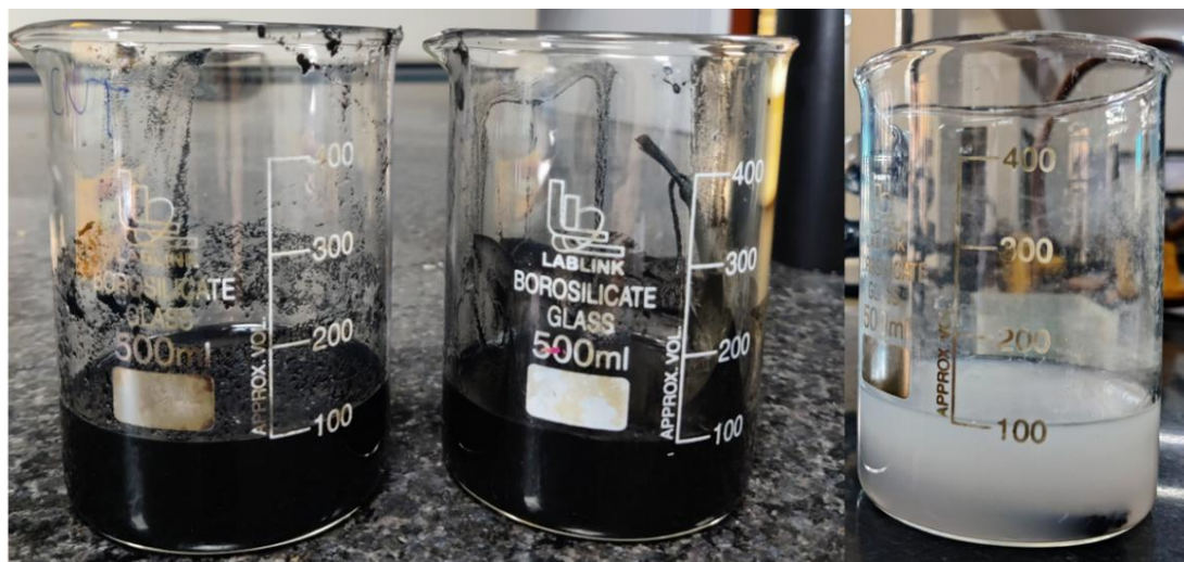
(a) (b) (c) Figure 3.5. Illustrates the nanospecies coating of (a) MWCNT (b) graphene (c) ZnO on the fiber
