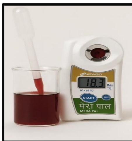
Figure 14: Measurement of total soluble solids (TSS) in cherry juice using a digital refractometer.
