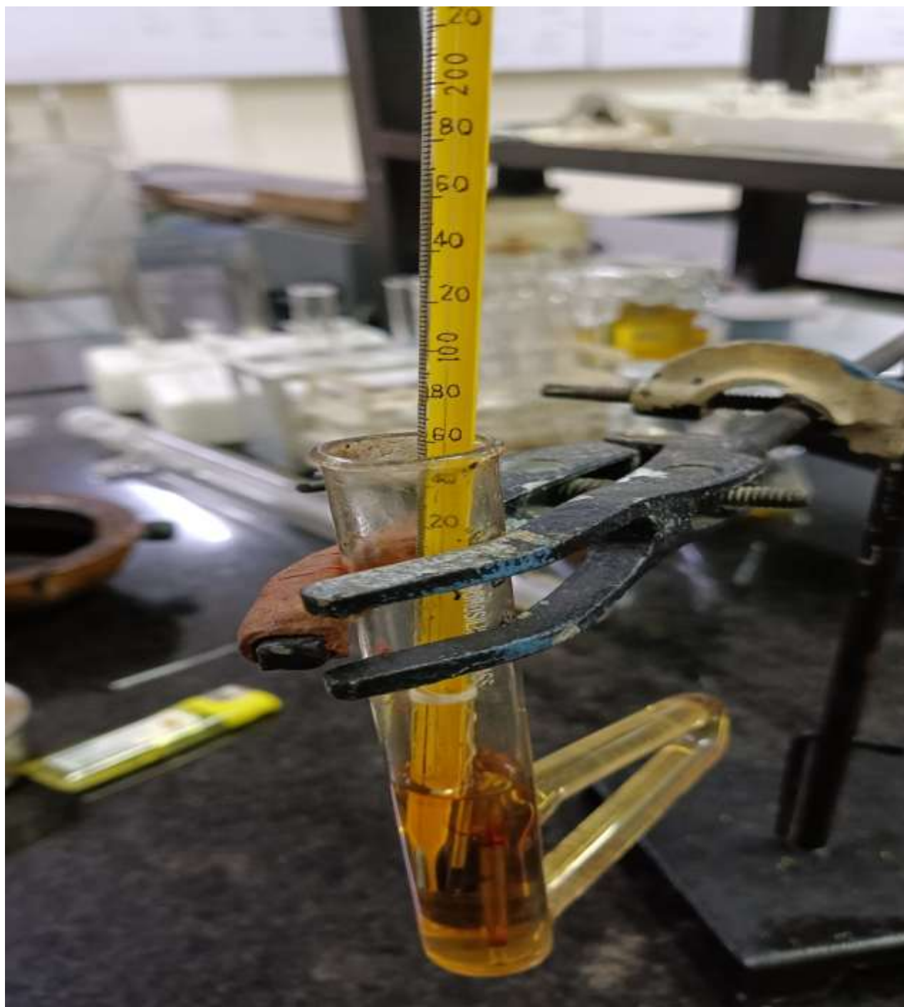
Fig. 5.4 : Melting point determination of Xn drug by Capillary fusion method
