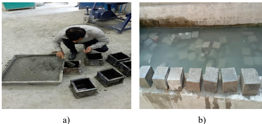
Figure 21: a) Casting of concrete Specimen b) Curing of the specimens in the curing tank
