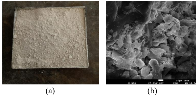
Figure 12: a) Sample of metakaolin used b) SEM image of Metakaolin particles
