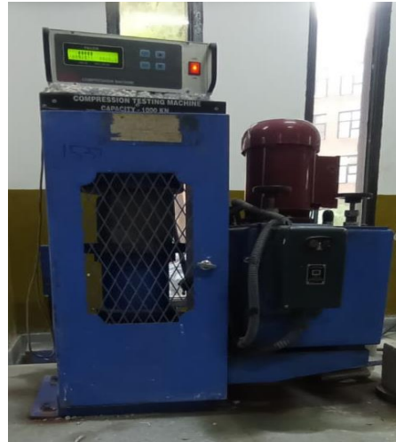
Figure 23: Compression Testing Machine (CTM)
