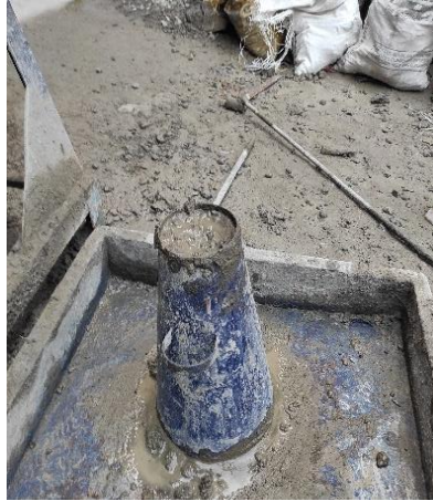
Figure 22: Slump cone for workability
