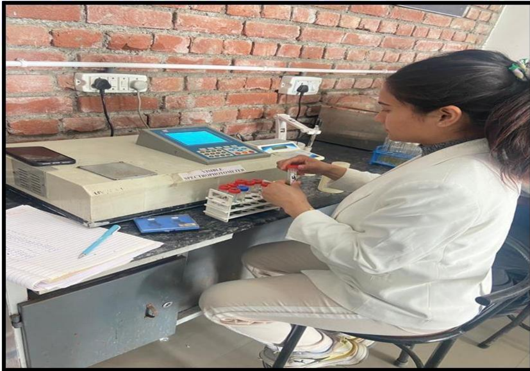
Image 17: Recording the optical density using a spectrophotometer
