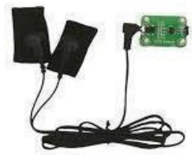
Figure 3.11: Galvanic Skin Response (GSR) Sensor (Source: https://www.theengineerstore.in/products/gsr-skin-current-sensor-v2-0 )
