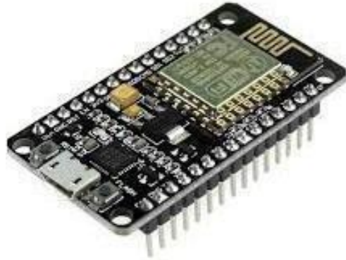
Figure 3.13: NodeMCU ESP8266 Module (Source: https://www.amazon.in/Generic-Nodemcu-Esp8266-Internet-Development/dp/B07262H53W?th=1 )
